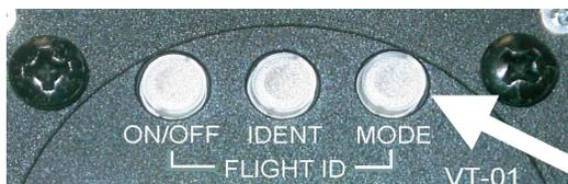
The current mode is shown in the centre of the bottom line of the screen. Pressing the mode key circulates through the following modes:
