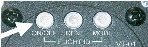
Press the On/Off key shortly to switch on the unit. After the system start, the screens shown below are displayed.
