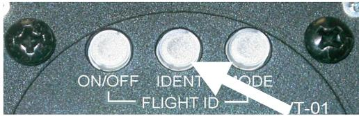
If required by ATC, press the IDENT key (middle of the 3 keys of the transponder)
